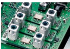
Hi-spec 1st IF filters (Roofing filters)
