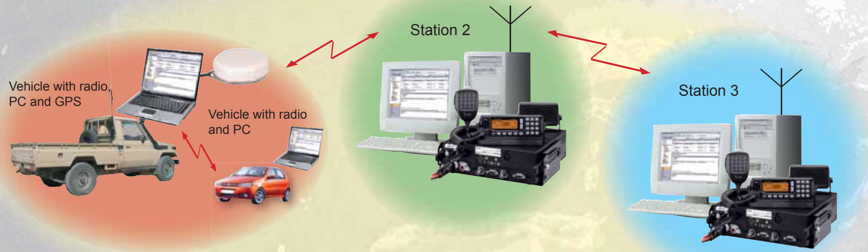
(a) Example of a network with radio-only communication access. The stations exchange emails by radio. A vehicle that has a PC can also send emails through the closed network, and even be localised if it is equipped with GPS.
